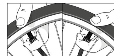
**9** If you are using tyre sealant: For inflation place the tyre with the valve at the 11 or 1 o'clock position. Otherwise sealant could leak into the valve or put too much turbulence into it. It could dry faster or lock up the valve core.
