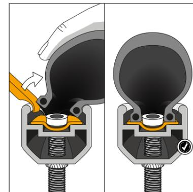
**4** Mount the Tubeless tyre on the rim in correct orientation of rotation. Ensure no loose pieces (e.g. sand, plastics) are found inside. Due to the tighter dimension tolerances of a tubeless tyre compared to a normal clincher tyre, it may be helpful to use tyre levers.
