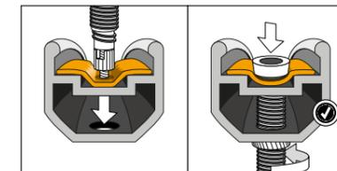
**2** Mount the Tubeless valve first. Install it from the inside of the rim and tighten the nut. Press your finger on the rubber end of the valve to secure a better fit. Only tighten the nut by hand, do not use any tools.
