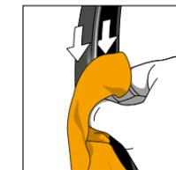
**3** Before the initial inflation you can apply some soapy-water or a mounting pad on the contact points between tyre and rim bed. This can help improve mounting the tyre on the rim.
