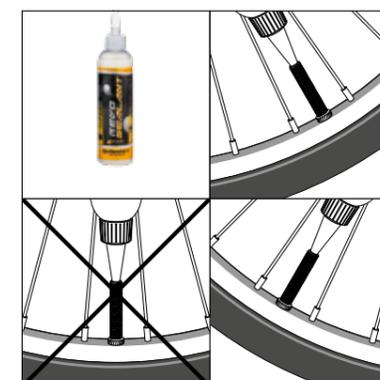
**8** For the best puncture resistance, we recommend to fill approximately 30 - 60 ml of tyre sealant through the valve. Considering it will dry over time, it is best to check and refill it every 3 - 6 months.
