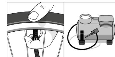
**5** To fit the tyre between the hooks, you may need a higher amount of air in the first instance. If you are using a floor pump, it is better to maintain a constant momentum within the first few seconds. A modern floor pump with a second inflatable cartridge can help to achieve this.
