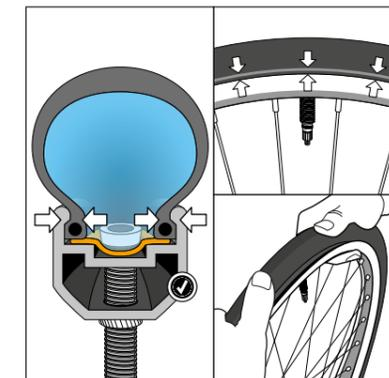
**6** The correct fitting of the tyre on the rim is mostly notable by a loud clicking noise. Check the air tightness of your Tubeless system. Does it lose any air? Check if the control line has an equal distance to the rim. If not release some air and work on the tyre with both hands.
