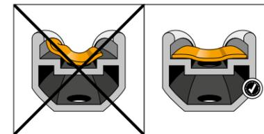
**1** Check both rim and rim tape. Only use Tubeless ready rims. Ensure that the rim tape covers the rim well with at least two layers.
