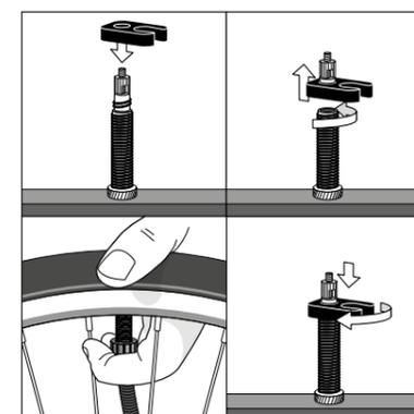
**7** To enhance the air volume, unscrew the valve core. Pump it up and screw the valve core in again.
