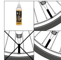
For the best puncture resistance, we recommend to fill approximately 30 - 60 ml of tire sealant through the valve. Considering it will dry over time, it is best to check and refill it every 3 - 6 months.
