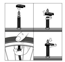
To enhance the air volume, unscrew the valve core. Pump it up and screw the valve core in again.
