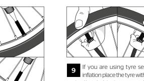
If you are using tyre sealant: For inflation place the tyre with the valve at the 11 or 1 o'clock position. Otherwise sealant could leak into the valve or put too much turbulence into it. It could dry faster or lock up the valve core.
