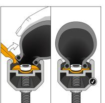
Mount the Tubeless tyre on the rim in correct orientation of rotation. Ensure no loose pieces (e.g. sand, plastics) are found inside. Due to the tighter dimension tolerances of a tubeless tyre compared to a normal clincher tyre, it may be helpful to use tyre levers.
