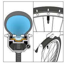
The correct fitting of the tyre on the rim is mostly notable by a loud clicking noise. Check the air tightness of your Tubeless system. Does it lose any air? Check if the control line has an equal distance to the rim. If not release some air and work on the tyre with both hands.
